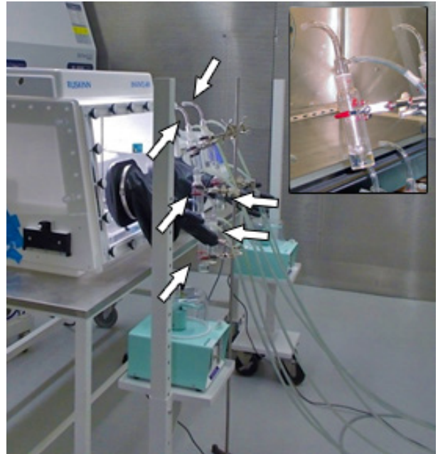
Figure 5: Six impingers were placed in the area where the user would typically work with the Invivo 2 . See top inset for a close-up of the glass impingers, similar to those used in this test.
