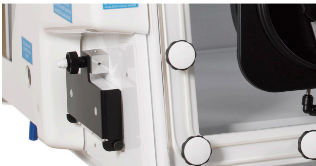
Figure 3: The SPES (shown above) is a mailbox-like slot that allows quick side entry or exit of individual plates and bypasses the interlock cycling process.
