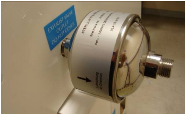
Figure 2: An in-line HEPA disc filter installed on the discharge side of the exhaust valve of the Invivo 2 workstation.
